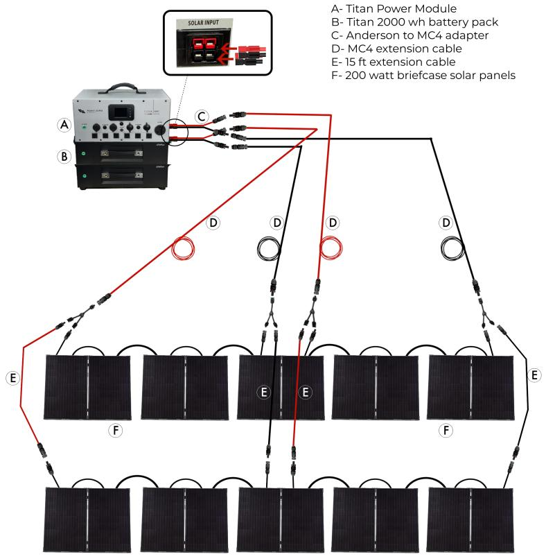
BEFORE CONNECTING SOLAR TO THE TITAN, check the voltage of your solar panels with the included volt meter while in direct sunlight. IF VOLTAGE IS OVER 120V, DO NOT CONNECT TO THE TITAN.
